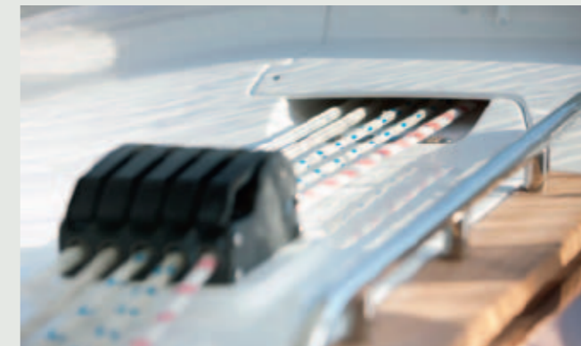
Halyards and sheets are guided into the cockpit, making them easy and safe to use.
