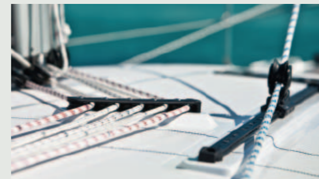
Genoa tracks, adjusted with precision to get the optimum position for the headsail.
