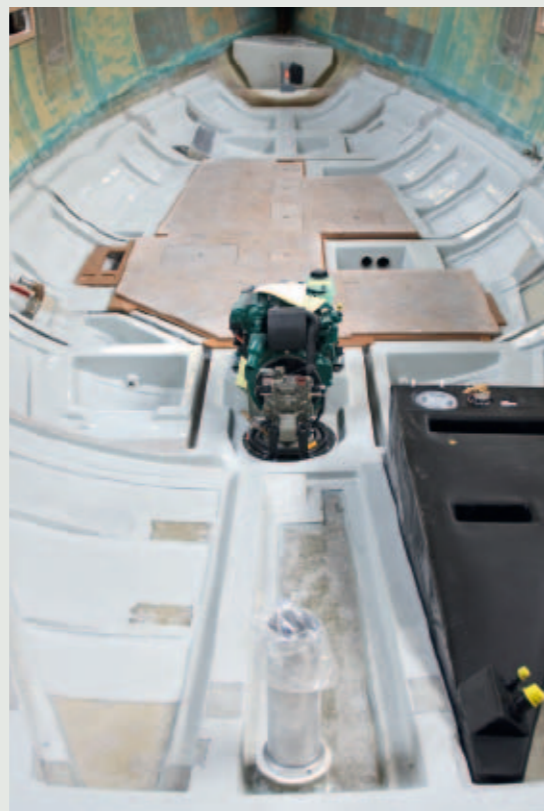
A stable floor assembly manages the forces of rig, hull, keel and rudder - all the chambers of the floor assembly are integrally linked.
